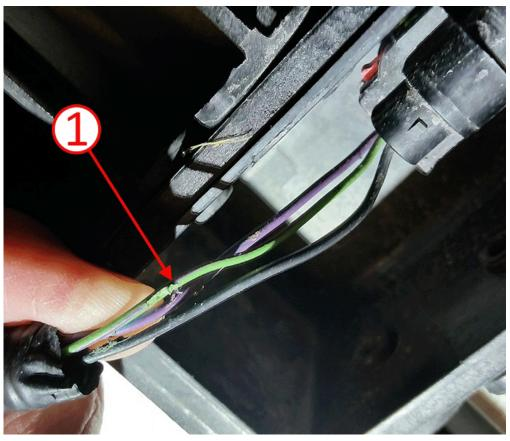
Inspect the active shutter wiring harness for any signs of chafing (1).
