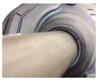
1. Remove the intermediate steering shaft boot (seal) (outer). Verify that the intermediate shaft boot bushing is completely contained within the rubber boor Refer to *Intermediate Steering Shaft Boot Replacement (Outer)* in SI.
