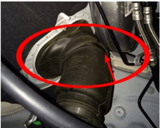
2. Remove the intermediate steering shaft boot (seal) (inner). Confirm that the bearing is properly seated inside the rubber boot. Refer to *Intermediate Steering Shaft Boot Replacement (Inner)* in SI.
