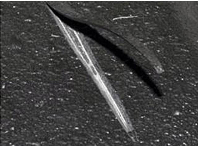
11. Long tears are handled in the same way but broken down into smaller sections to allow enough time to complete the section within the cure time of the material and to be small enough to be covered by the textured pad.
