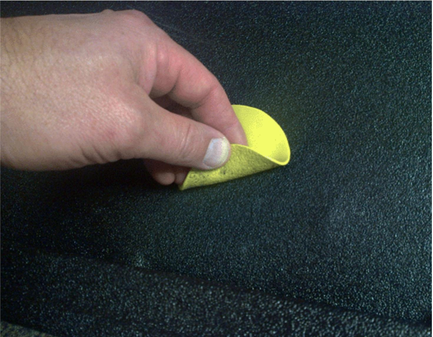
9. Release the pressure and slowly remove the pad. If any material sticks to the pad, it can be removed once dry.
