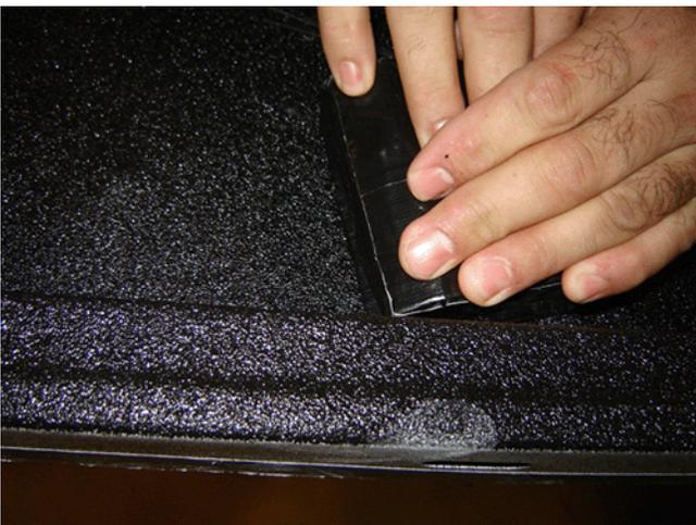
8. Using a small block, such as a piece of 2 x 4 wood, allows for a more even pressure application.
