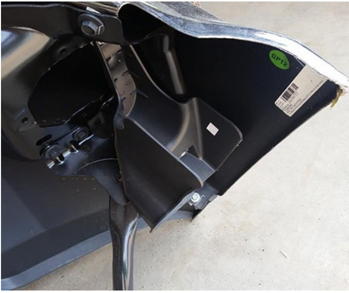
OEM bumper with intake air box protection to help prevent moisture and other debris getting into the air cleaner box.
