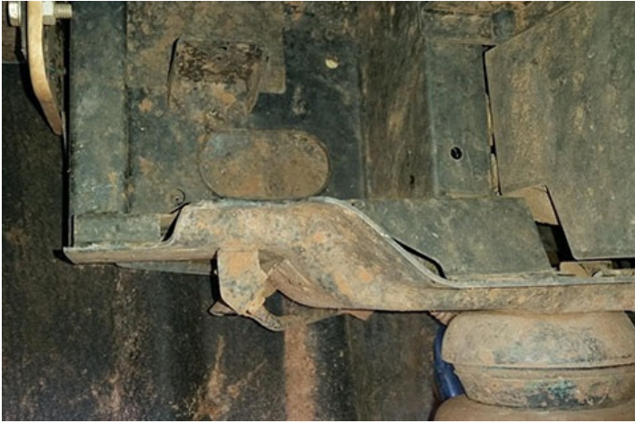
Aftermarket bumper without intake air box protection.
