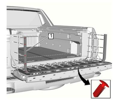
7. Using a trim type tool, release and remove the five driver's side endgate weather-strip (1) retainers.
