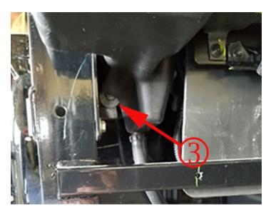
18. Remove Cargo Box Stowage Box Bracket Bolt in Stake Pocket (3)
