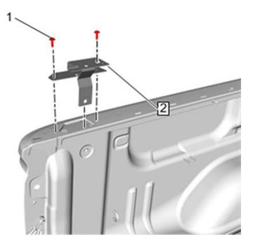
17. Remove two Cargo Box Stowage Box Bracket Bolts (1)
