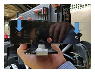
19. Elongate holes in Cargo Box Stowage Box Bracket (1) and (2) to allow bracket to be moved forward (towards the front of vehicle). This allows the trim to move forward and allows the holes to line up for remounting of the trim.
