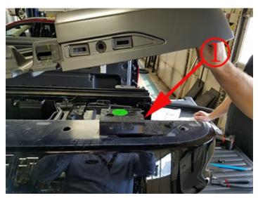
16. The Upper panel should now be loose. Raise and support panel to expose mounting bracket.
