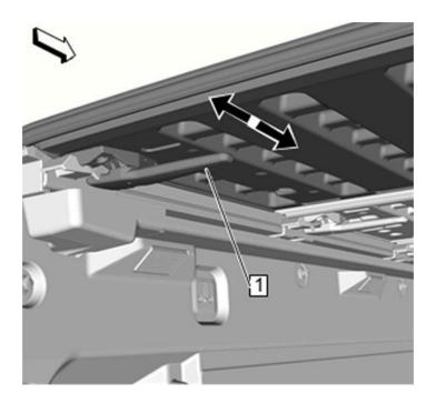
2. Remove each cargo cover by pulling the handle on the left and right side of each cargo cover.
