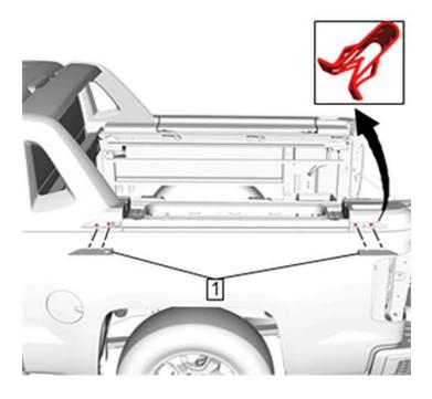
12. Using a trim type tool, remove the pickup box side upper molding (1)
