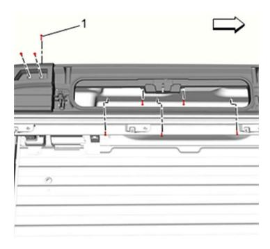
15. Remove eight Pickup Box Side Upper Molding Bolts (1)
