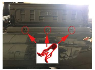
13. Using a trim type tool, remove the pickup box side center molding (there are 3 retainers and two sided tape securing the molding.)14. Clean the area with a 50/50 mixture by volume of isopropyl alcohol and clean drinkable water to remove any leftover adhesive residue.
