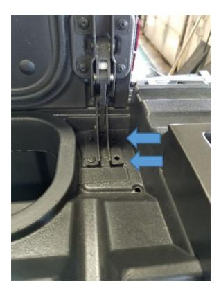
11. Remove Tool Box Lid Hinge Spring Bolt (1) Note: Only remove outer screws only [4x]. This prevents mis-alignment of the door upon re-assembly
