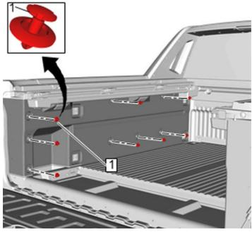
6. Remove eight Pickup Box Side Liner Retainers (1)
