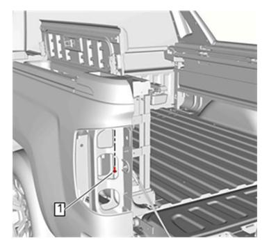
10. Remove Pickup Box Molding Bolt (1)
