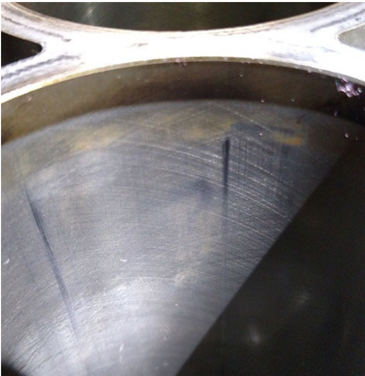
Shown below is an example of a damaged cylinder wall. In this example the scuffing is wide and has removed the crosshatch from the cylinder wall in the area above the arrow. This would result in oil consumption and requires engine replacement.
