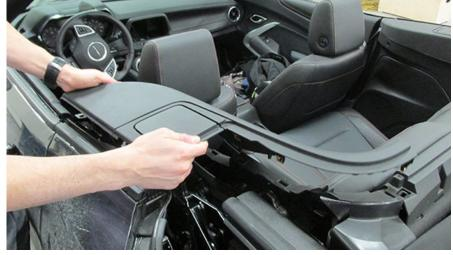
If the noise is narrowed down to the "flipper doors", replace the entire trim panel. Concern #2
