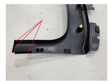
Once this has been verified, dealership technicians should also verify that all six foam blocks are present, and are located in the correct areas. The photo below should be used as a guide to verify the blocks are in the correct location. If any of them are missing or damaged, relocate or replace them as needed.
