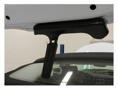
• The second area of concern may be the metal receiver that the alignment pin slides into. Remove the receiver from the vehicle, as seen in the photo below, and place it on a flat work surface.
