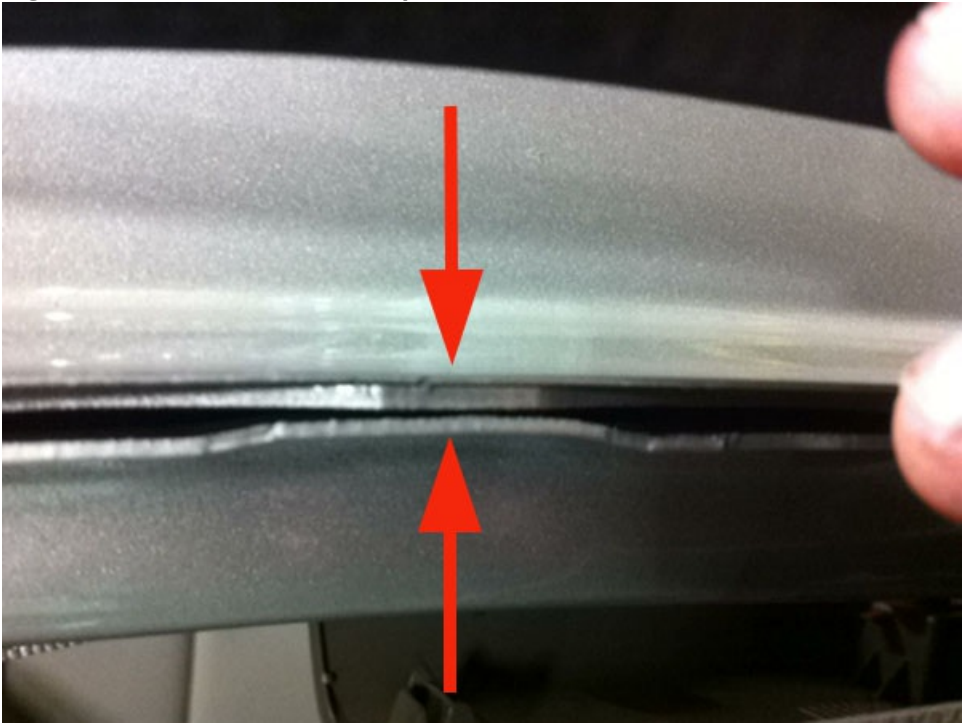
Repair welds as necessary Condition 2: Inspect B pillar in area near seat belt mounting where there are three pieces of sheet metal sandwiched together for contact between the panels.
