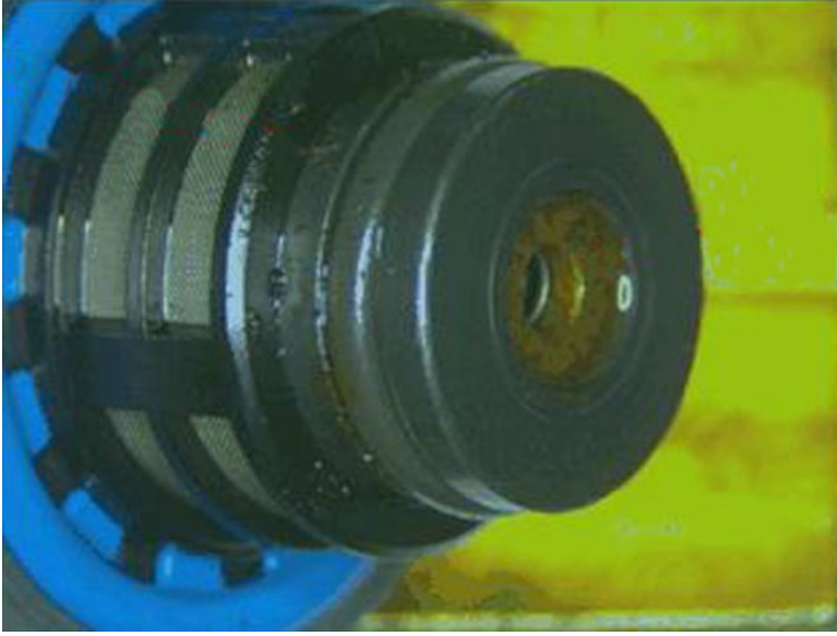
Fuel Pressure Regulator 1 With Rust Due To Water Contamination
