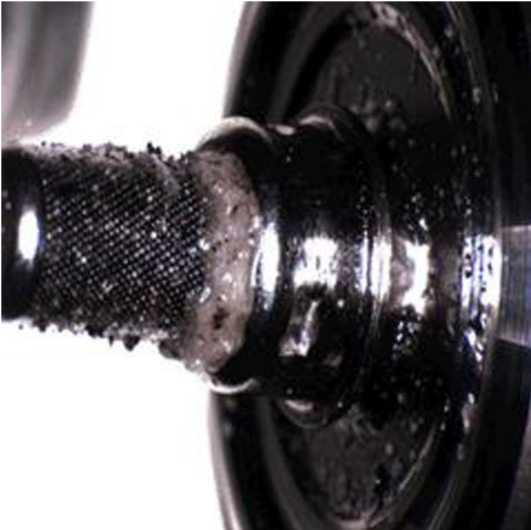
Fuel Pressure Regulator 2 With DEF Contamination
