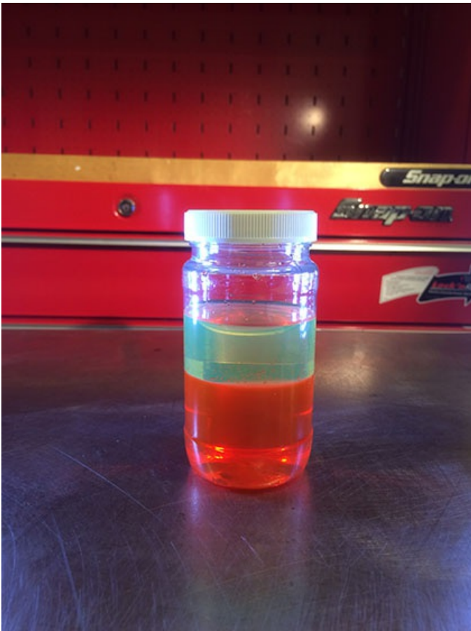
Diesel Fuel and Coolant
