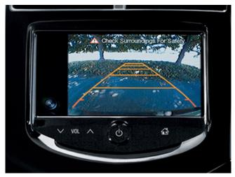
Some customers may comment that when using the rear vision camera, it only shows on 3/4 of the radio display screen.
