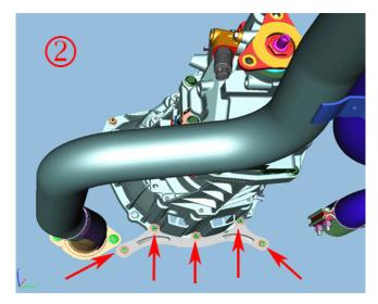
Inspect the M8 nuts that secure the catalytic converters to the exhaust bracket. RPO LF3 (1) and RPO LF4 (2) as shown above. If the nuts are loose, it is necessary to replace them with new torque prevailing nuts.
