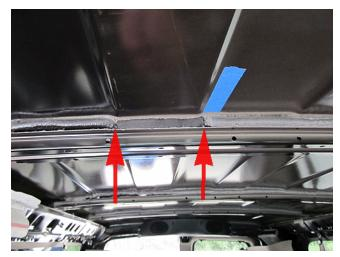
8. Install the 7/16 in. thick material between the roof panel and the third roof bow as shown. Ensure the material is positioned toward to the center of the roof bow.
