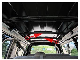
2. Locate the third and fourth roof bow (counting from the front of the vehicle).
