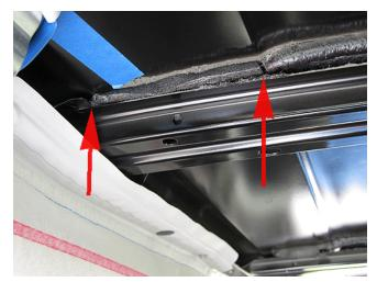
7. Install the 5/16 in. thick material between the roof panel and the third roof bow as shown. Ensure the material is the position closest to the outer end of the roof bow.
