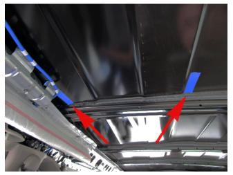
**3.** Mark the section shown with masking tape.
