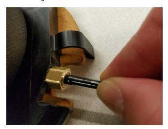
2. The airline should continue to be inserted until it bottoms out and can no longer be inserted any further.
