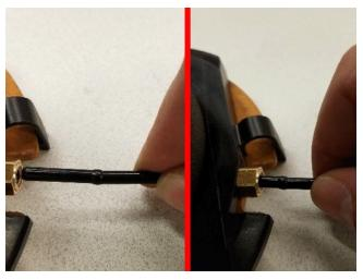
1. The airline should be inserted until resistance is felt in the system. The photo above shows how far the line must be inserted before the resistance begins.
