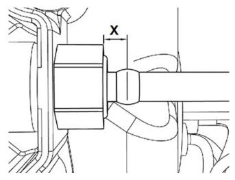
The air suspension system is very robust and if a vehicle is reported to have an air suspension failure in the first 5000 miles (8000 km), it is likely the the airline connections at the air springs were assembled incorrectly during the manufacturing process. The design of the airline does not allow for to be partially inserted. It will either be fully seated or sitting loose in the fitting. There should be about 3-4 mm from the face of the valve to the note the airline (Dimension X above).
