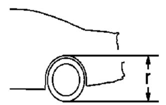
R Height: The vertical distance from the ground to the top of the wheel opening through the center line of the rear wheel.
