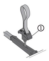
Replace both original quarter turn tonneau latches with new design spring latches (1) from the appropriate parts kit listed in the Parts table.
