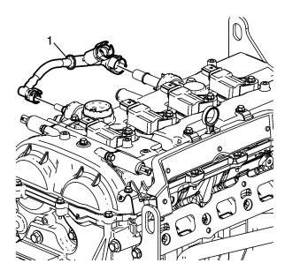
Replace the positive crankcase ventilation hose assembly. Refer to Positive Crankcase Ventilation Hose/Pipe/Tube Replacement in SI.
