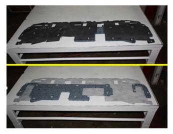
• If the vehicle contains the 2D insulator shown in the front and rear view examples above, acoustic performance can be gained by replacing the insulator with the 3D design. Replace the body rear panel insulator. Refer to *Body Rear Panel Insulator Replacement* in SI.
