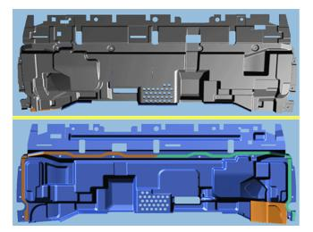
• If the vehicle contains the **3D** insulator shown in the front and rear view examples above, DO NOT replace the insulator. No further repairs ar recommended.
