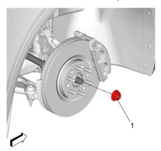
**Caution: DO NOT** use air tools to remove the wheel drive shaft nut. Damage to the wheel drive shaft threads could occur. Use hand tools only.
