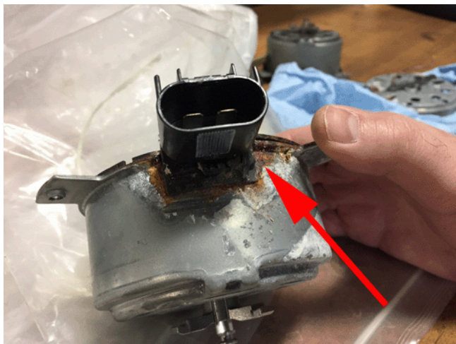
Note: Metal fan motor housing with corrosion (not OK)
