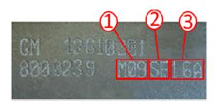
If the vehicle exhibits this condition, remove the starter assembly and inspect for date code correlating with build on date 09/16/2016. The code pictured above shows the day (01), month of September (2) and the year (3).
