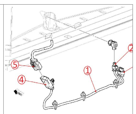
Inspect the ambient air temperature sensor wiring harness connectors B9 (2), M60B (3) and the X119 (4, 5) for any signs of corrosion.
