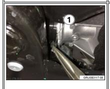
Insert a 3mm feeler gauge (3mm drill bit shown) into the gap between the output shaft and the extension housing (1). If the feeler gauge fits tight or will not fit (gap is ≤ 3mm) then no further repair is necessary. If the feeler gauge fits loose (gap >3mm), replace the output shaft. Follow Repair Instruction 31 60 000 Removing and installing/replacing left or right output shaft. (Right Side - KSD2: 31 60 504)
