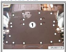
Remove the center lower protection cover (1). Tightening torque of screws when reinstalling is 3Nm.
