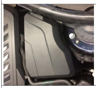
3j.Replace the cover of the DME control unit. Ensure the repaired harness is not pinched, rubbing on a sharp edge, and is fully covered by the DME control unit cover.
