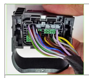
2d. All slots in the connector must be occupied with a wire or sealing plug.
