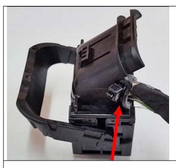
2a. Remove the cable strap (arrow) on connector A368\*1B.
