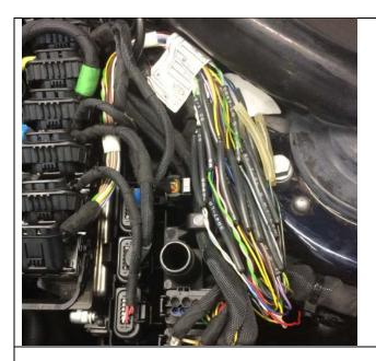
3e. Using the supplied butt connectors, splice in the replacement wiring harness, one wire at a time, using the black shrink tubing.
