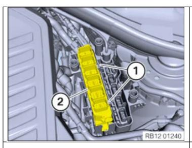
3h.Unlock clamps (1) and remove the DME control unit (2) towards the top.
