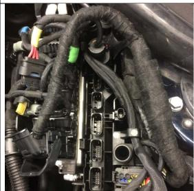
3f. Wrap the wiring harness with repair tape (P/N 61 13 6 920 760) up to the connector.
