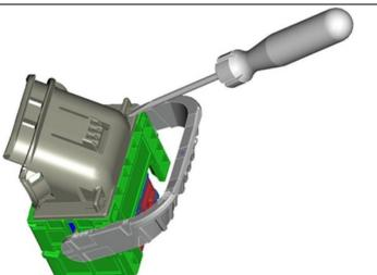
3c. Carefully remove the protective cap from the connector using a suitable tool on both connector A368\*1B and the repair harness.
