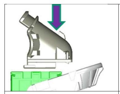
2g. Attach protective cap and replace cable strap
