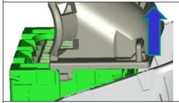
Lift the protective cap off the connector
