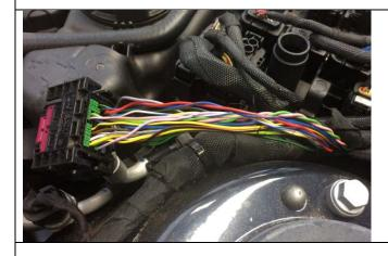
2c. Remove approximately 4" of the insulating tape on the wiring harness from connector A368\*1B
