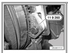
After removing of the transmission, secure the flywheel using the special tool 119 260.
