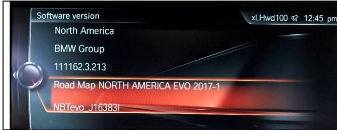
8. Check and confirm that the installed road map version is the identical road map version which was installed in the defective HU
