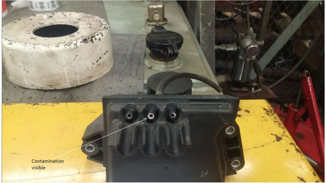
Vacuum reservoir contaminated output ports.jpg:
