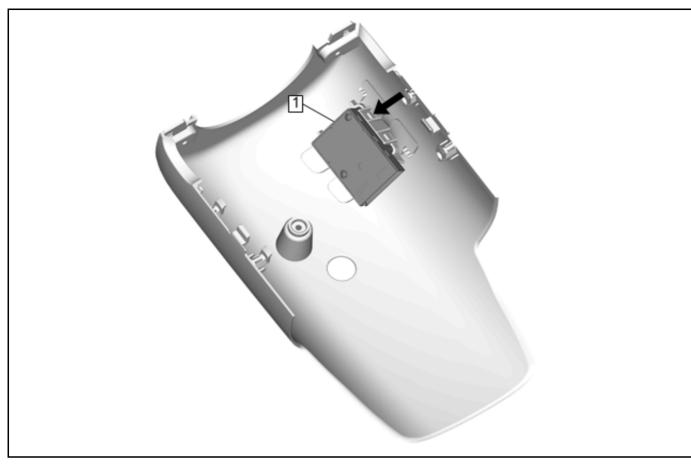
3. Apply butyl tape around sides of switch pocket to hold the retention clips against the switch.
