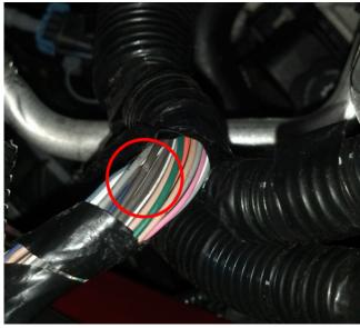
If no damage is found, wrap Woven Polyester Electrical Tape (PET) (preferred) or equivalent anti-abrasion tape around the wires on the harness.
