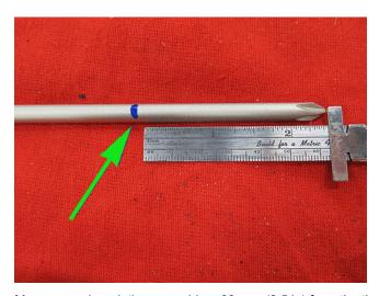
2. Measure and mark the screwdriver 63 mm (2.5 in) from the tip as shown.
