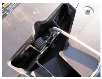
4. With release lever depressed, rotate the release tool to the right (towards driver's side) releasing the hood lock.
