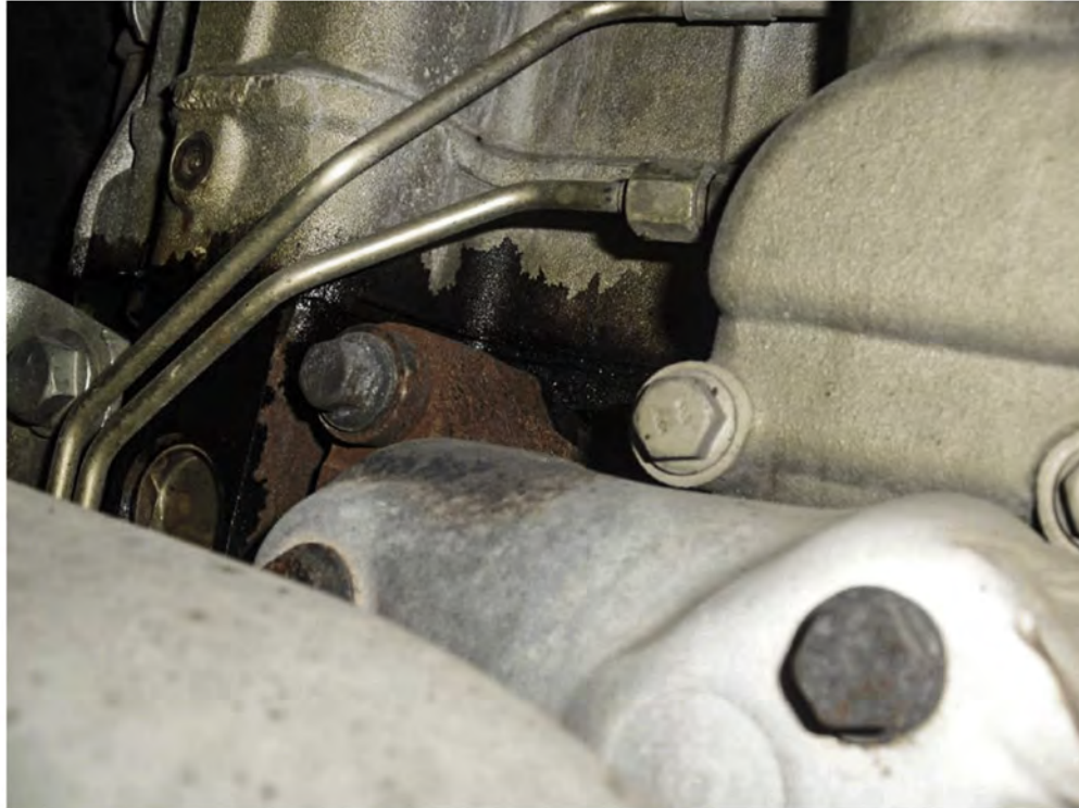
Figure 3. Example of an Oil Leak: Very Wet with Evidence that Fluid Leaks onto the Ground
