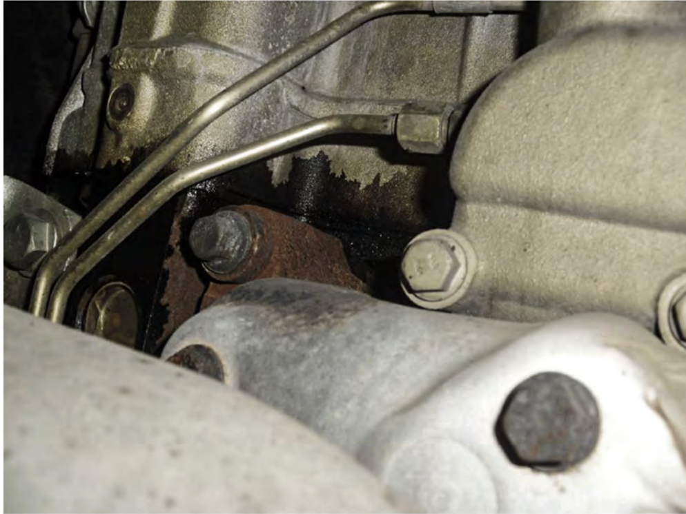
Figure 7. Example of an Oil Leak - Very Wet with Evidence that Fluid Leaks onto the Ground
