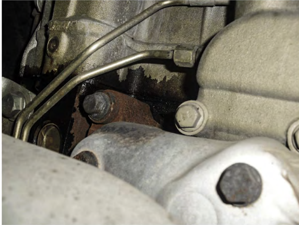
Figure 1. Example of an Oil Leak - Very Wet with Evidence That Fluid Leaks onto the Ground
