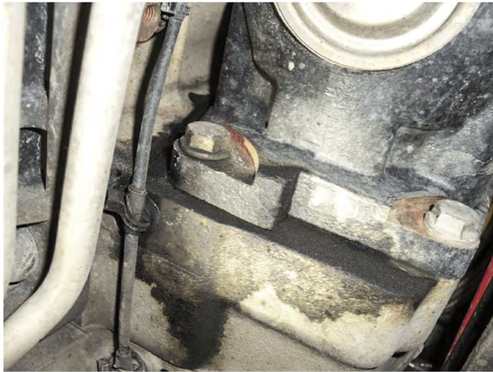
Figure 8. Example of a Seep - Residue Accumulation on the Surface but Remains on that Surface and Does Not Drip onto the Ground
