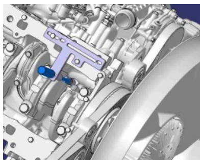
Figure 21. W936589016100 – Piston Cooling Nozzle Tool
