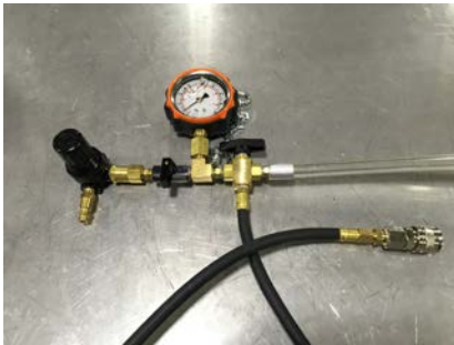
Figure 28. DSN930E16010 – Low Pressure Leak Test Tool
