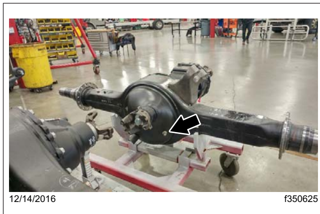
Fig. 6, Forward Rear Axle Fill Location
