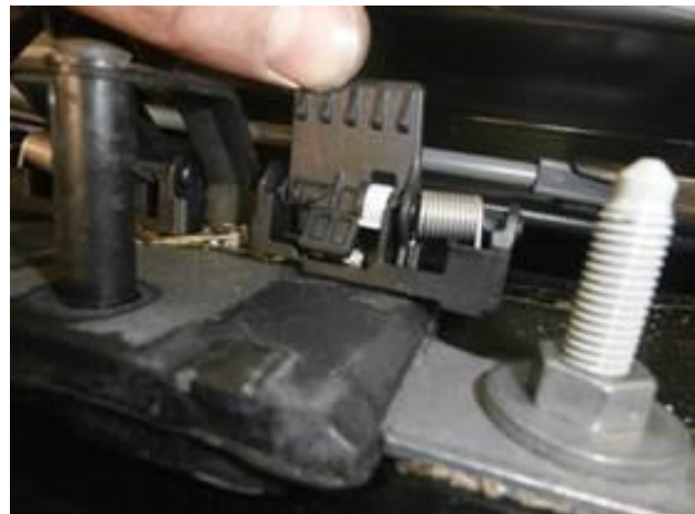
Figure 5. Debris trapped in the Rear Lid Closed Sensor.
