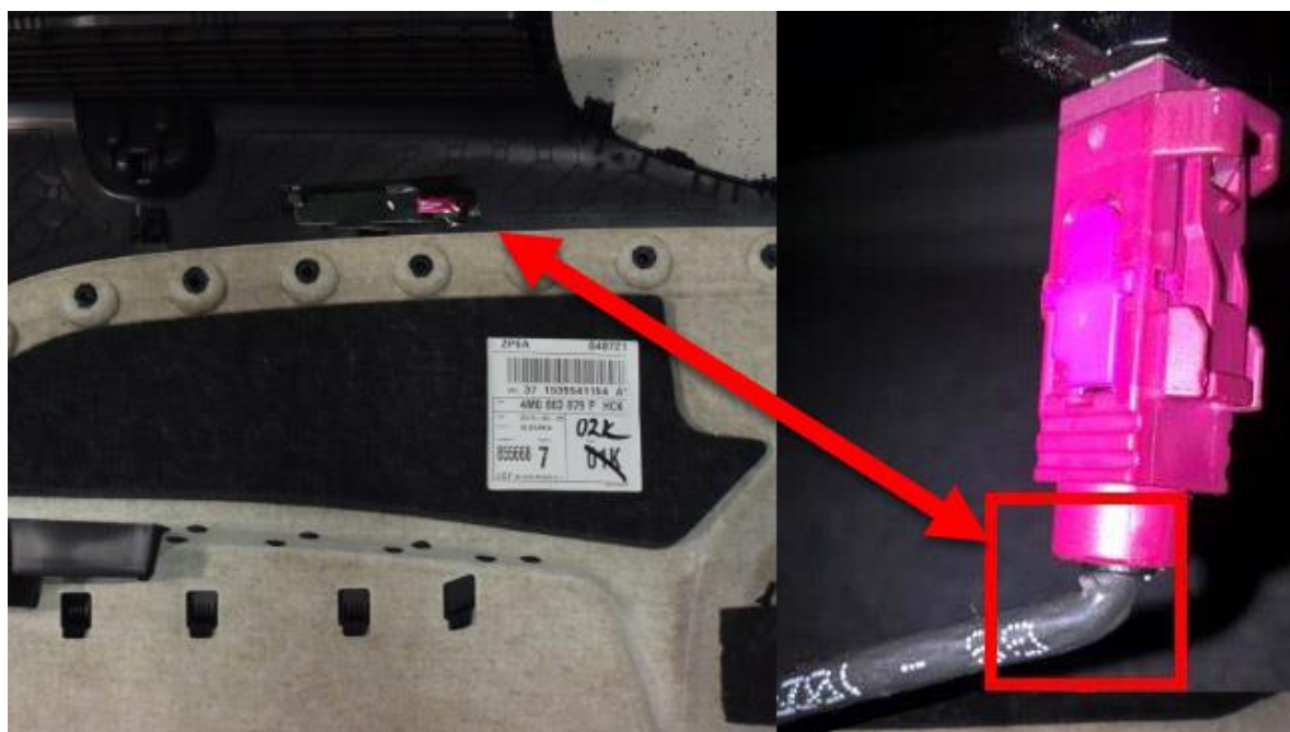
Figure 2. Coaxial wire kinked at R263 SOS Antenna.
