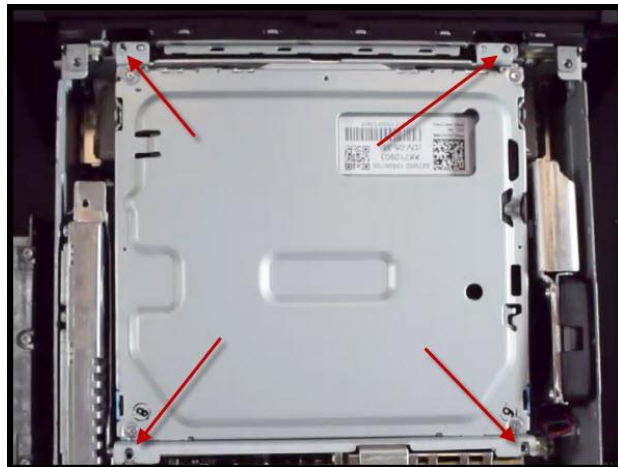
Figure 9. CD drive mounting points are free to move.
