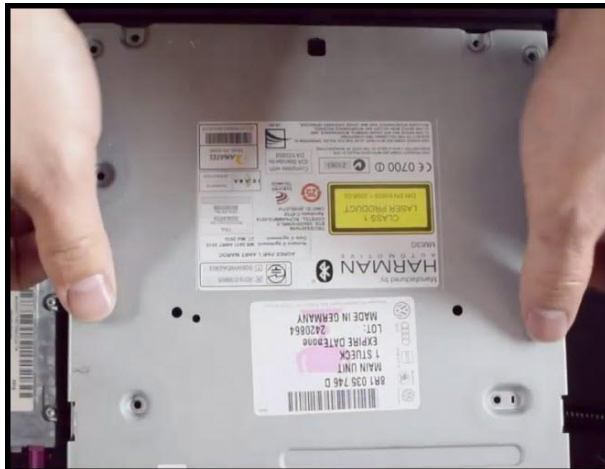
Figure 7. Pry top cover off with fingers.
