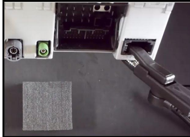
Figure 4. VAS6613 ESD work surface grounding device clip.
