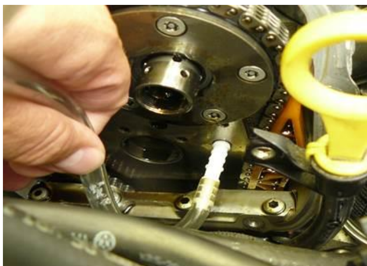
Figure 7. Press pressure line with adapter of VAS 6213 firmly into oil duct hole
