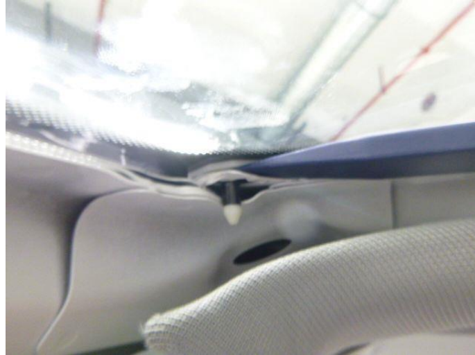
Figure 1. Increase the distance between plastic pin and metal lug.
