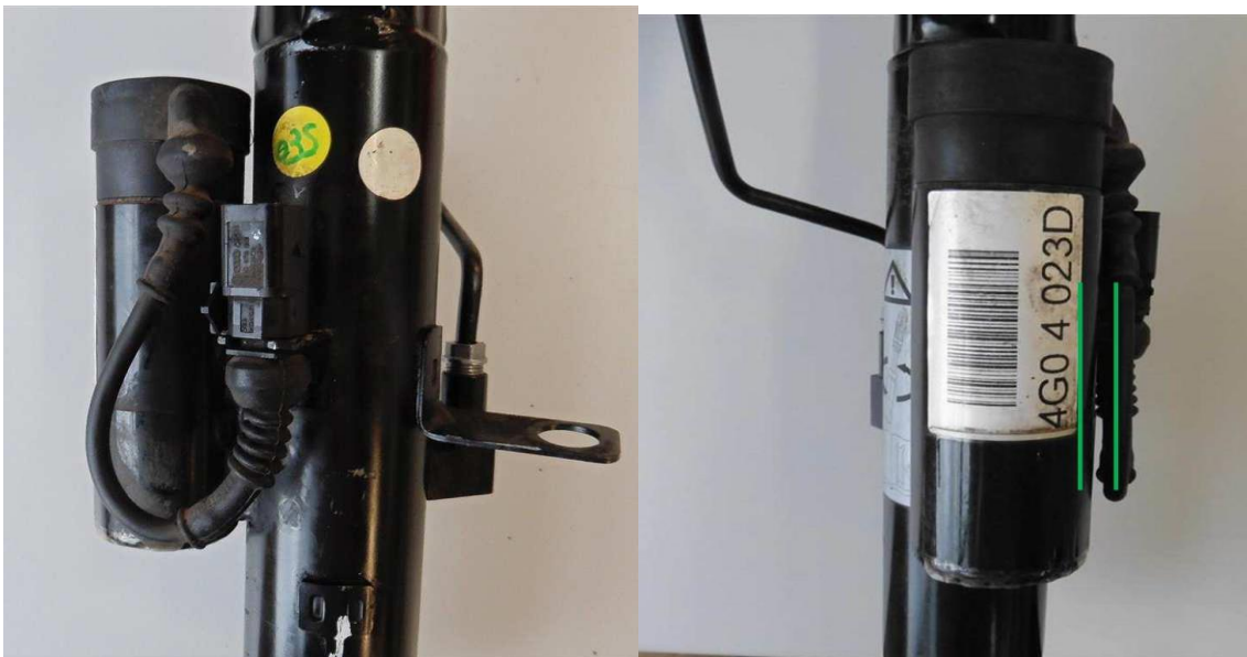
Figure 2. Correct connector alignment and cable routing.
