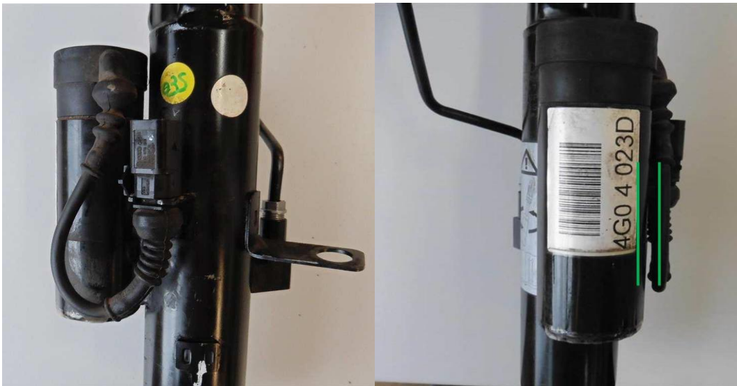
Figure 2. Correct connector alignment and cable routing.
