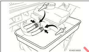
h) Slide back the 2 hose clips, disconnect, and immediately plug the 2 reservoir hoses.
