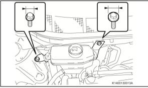
i) Reinstall the reservoir bracket with the 2 bolts.
