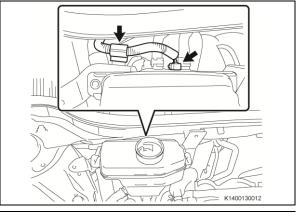
c) Detach the harness clamp and disconect the connector.
