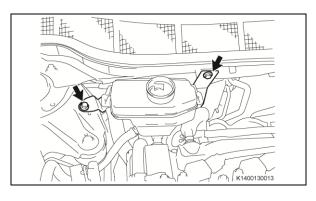
b) Remove the 2 bolts, and separate the reservoir bracket from the brake reservoir.
