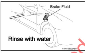
b) Brake fluid damages paint. **DO NOT** allow brake fluid to contact any painted surface. If brake fluid adheres to a painted surface, immediately rinse it off with water.
