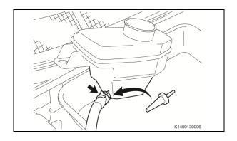
f) Slide back the hose clip, disconnect, <u>and immediately plug</u> the brake actuator hose.
