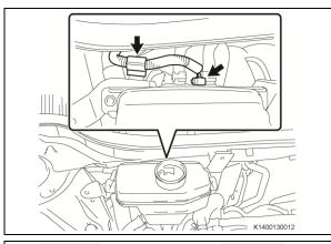
h) Reconnect the connector, and attach the harness clamp to the reservoir bracket.
