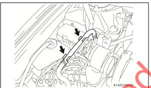
d) Detach the brake actuator hose from the 2 clamps.
