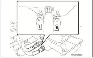
g) Apply tape and mark the resorvoir hoses to distinguish between left and right.
