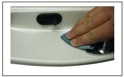
c. Using 3M General Purpose Adhesive Cleaner (P/N 08984) or equivalent, wipe down the affected area completely to remove all remaining residue of the original Certification Label.
