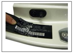
b. While continuing to apply heat, peel the label using a plastic scraper. Take caution to prevent damaging the paint.
