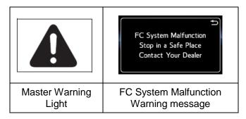
If the condition occurs during vehicle refueling, the master warning light flashes, the electric assisted power steering is disabled, the electric power steering system warning light comes on, the warning message of "FC System Stopped – Steering Power Low" is displayed on a Multi-Information Display, and a buzzer sounds.
