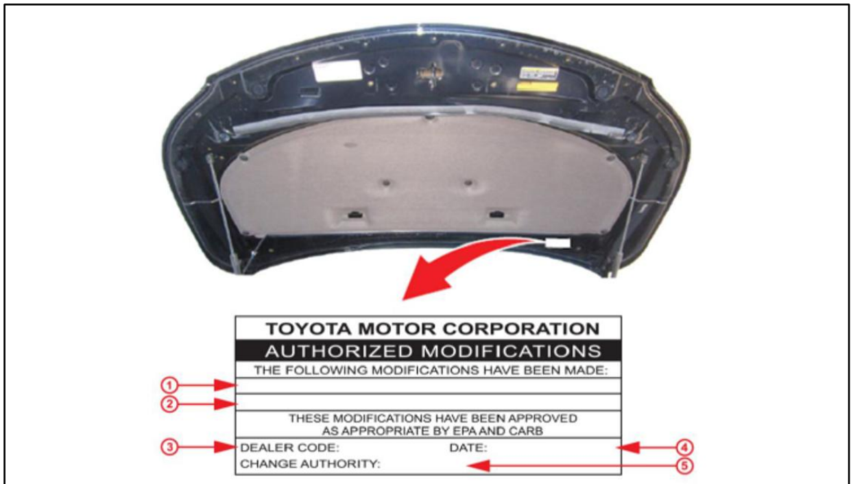
Figure 1. Location of Authorized Modifications Label for 2017 Sienna
