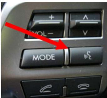
There have been reports of the Bluetooth pairing procedure not starting after pressing the talk switch on the steering wheel.
