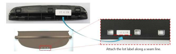
**4.** Assemble the new handle on the tonneau cover starting with the bottom half. Align the 3 connecting points with the 3 holes in the cover.
