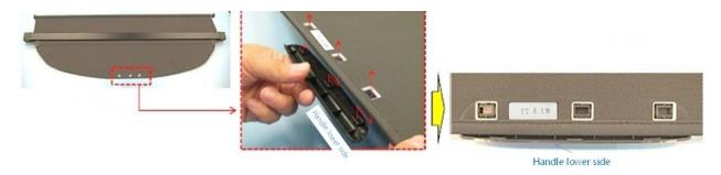
**5.** Align the upper half of the new handle with the 3 lower half connecting points. Use the center point as a reference for proper location.
