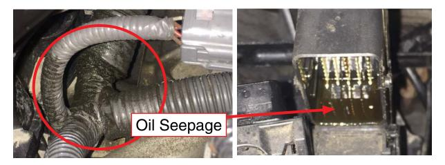
If related engine wiring harnesses and / or connectors are contaminated, the harness itself may also need to be replaced if degreasing affected components using a spray parts cleaner is unsuccessful.
