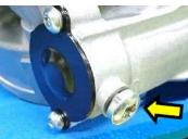
**Step 3-** Remove the tension spring and replace with the new part. Make sure the new spring is fully seated in the hole.
