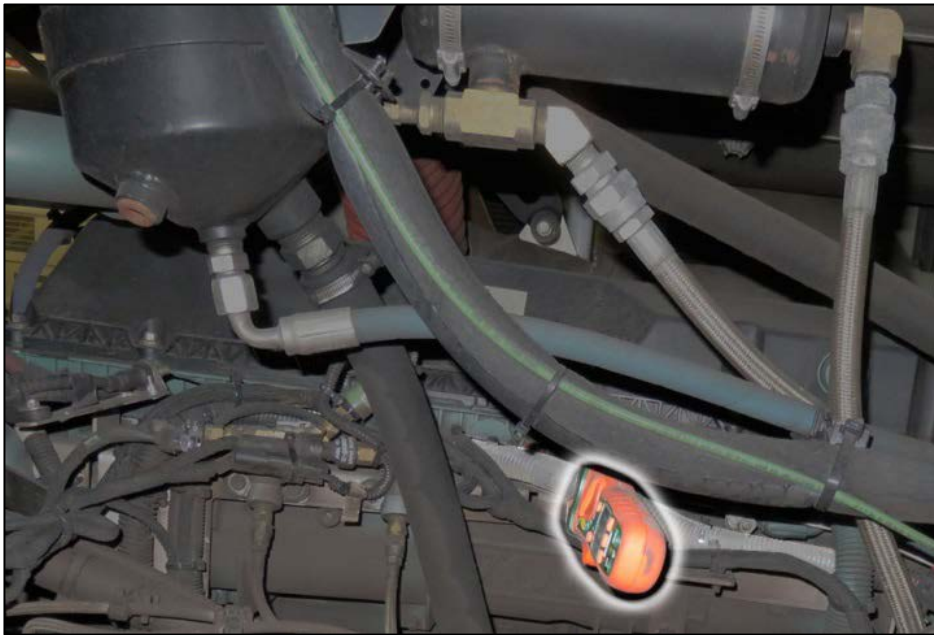
Figure 29: Main alternator cable suggested ammeter clamp position alongside engine.
