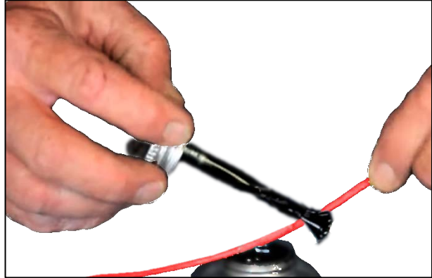
Figure 7: Liquid Tape Application
