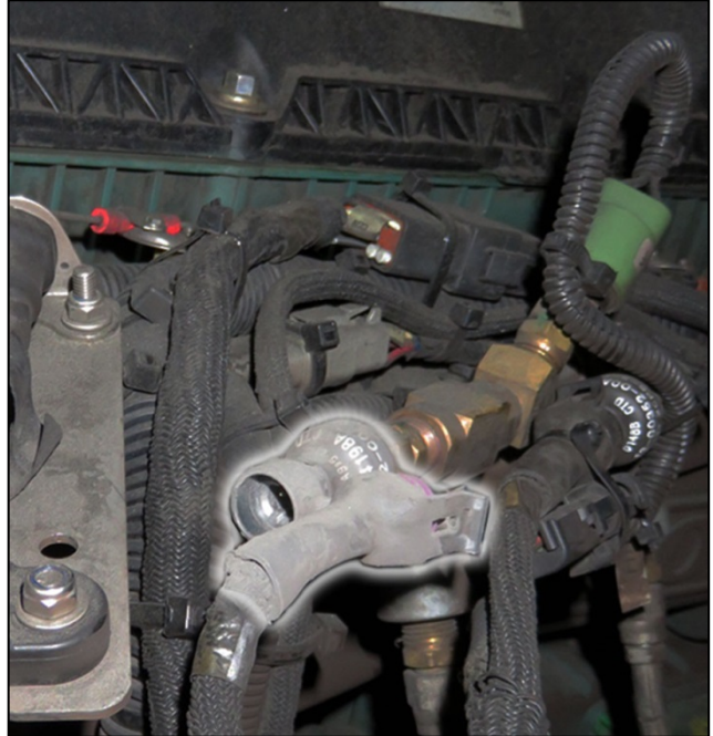
Figure 27: Disconnect Hi-side pressure transducer
