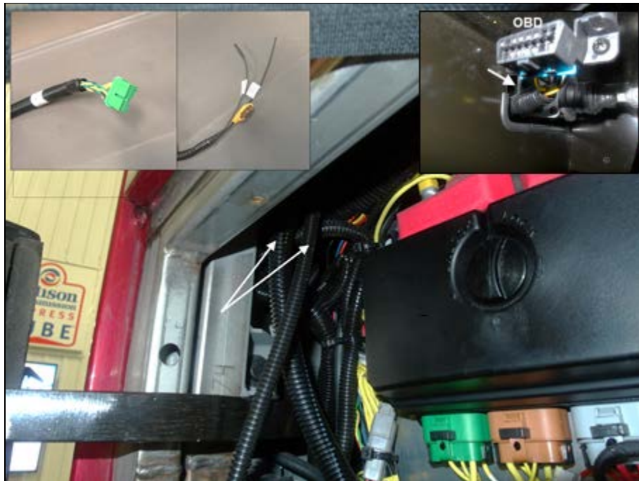
ELD HARNESS -MODULE CONNECTOR & POWER WIRES (H3 SHOWN)
