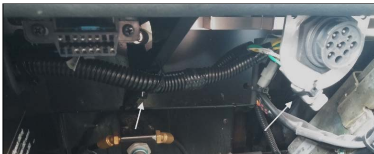
SECURE HARNESS UNDER DASH
