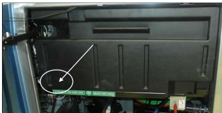
CHECK FOR INTREFFERENCE - INSIDE PANEL & MODULE HARNESS
