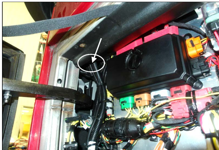
AVOID CONTACT HERE ON H3 VEHICLES
