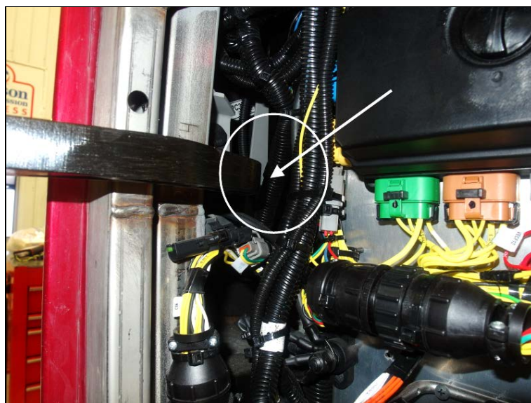
CHECK FOR CONTACT BETWEEN HINGE AND HARNESS (H3 SHOWN)
