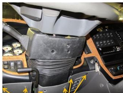
Screws Close-out panel
